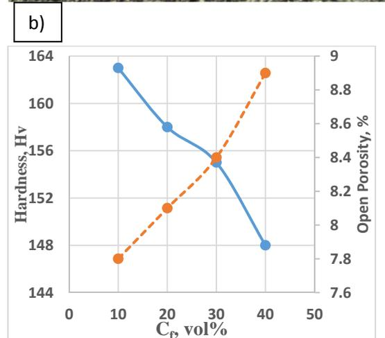
Fig. 4 Effect of  $C_f$  on hardness
