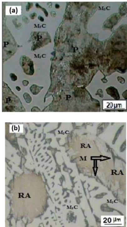
**Fig. 1 Optical metallographs of (a) conventional white cast iron (2% nital); and (b) alloyed white cast iron (Glyceregia - Marble). Eutectic carbides, pearlite, martensite and retained austenite are represented by M<sub>3</sub>C, P, M and RA symbols, respectively**
