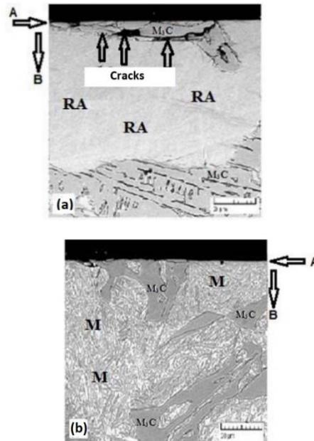
**Fig. 3 SEM images from the cross section perpendicular to the wear test surfaces of alloyed white cast iron samples showing the microstructural changes by stresses and mechanical forces at loads (a) 100N, and (b) 140N. Directions of A and B were represented to the parallel and perpendicular direction to the wear test surfaces, respectively. Eutectic carbides, martensite and retained austenite are shown by M<sub>3</sub>C, M and RA symbols, respectively**
