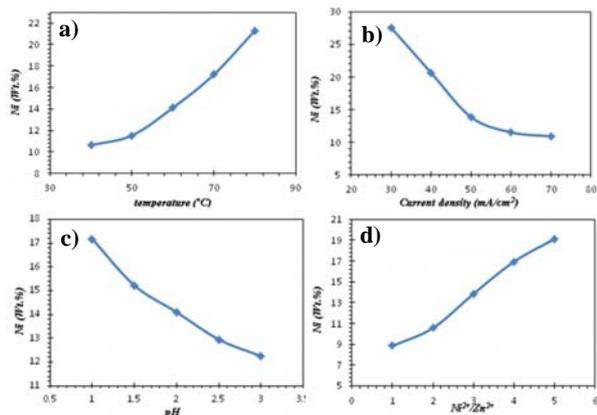
Fig. 1 Plot of Ni content vs. a) the electroplating bath temperature, b) the current density, c) the electroplating bath pH, d) Ni<sup>2+</sup>/Zn<sup>2+</sup> ratios in the electroplating bath
