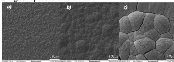
Fig. 5 Morphology of the Ni-Zn coatings deposited from baths with Ni<sup>2+</sup>/Zn<sup>2+</sup> ratios of a) 1; b) 2; and c) 5
