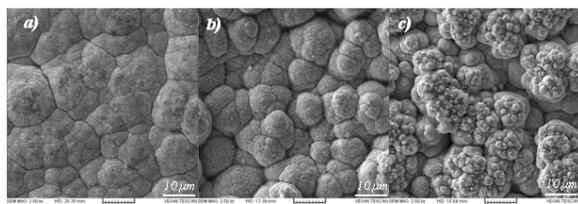
Fig. 3 Morphology of the Ni-Zn coatings deposited at current densities of a) 20; b) 40; and c) 60 mA/cm<sup>2</sup>
