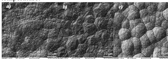
Fig. 2 Morphology of the Ni-Zn coatings deposited at a) 40, b) 60, and c) 80 °C
