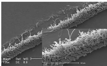
Fig. 3 TEM image of cross-section of scaffold (thickness)
