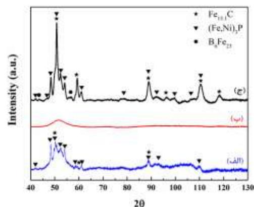
Figure 1. XRD pattern of  $(\text{Fe}_{1-x}\text{Ni}_x)_{77}\text{Mo}_5\text{P}_9\text{C}_{7.5}\text{B}_{1.5}$  ( $x=0.05, 0.1, 0.15$ ) samples
