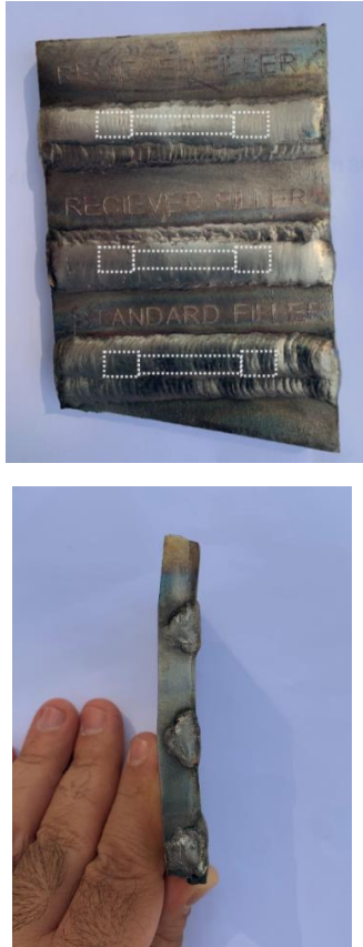
Figure 1. Weldments and the schematic of the tensile samples cut from the weldments
