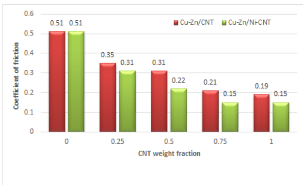
Fig 2 Coefficient of friction of uncoated and nickel coated CNT based copper nanocomposites at sliding speed of 0.3 m s -1 .
