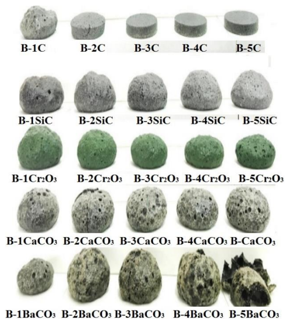
Figure 3: Images of the composite sample containing carbonate and carbon
