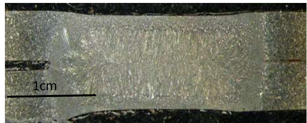
Figure 2. Macro-structure of welding sample of similar junction M/M
