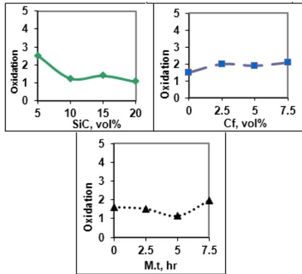
Fig. 2. The effect of SiC, Cr and M.t on oxidation
