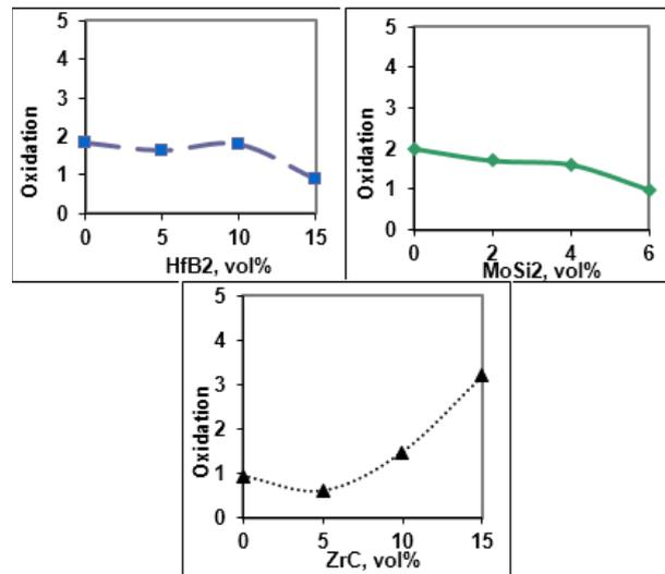
Fig. 3. The effect of MoSi<sub>2</sub>, HfB<sub>2</sub> and ZrC on oxidation
