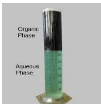
Fig. 2. Settler of stripping after first continues test
