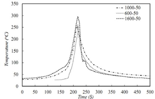
Fig. 1 Temperature-time diagram (thermal cycle) of the welding samples at velocity of 50 mm/min and rotating speed of 600, 1000 and 1600 rpm
