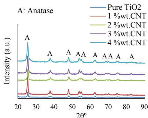
Fig. 1 XRD patterns of TiO<sub>2</sub>: MWCNT thin films
