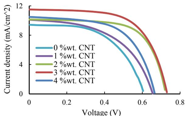
Fig. 4 Current density-voltage curves of DSSCs fabricated of TiO<sub>2</sub>:MWCNT anodes
