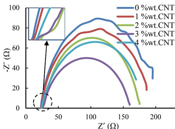
Fig. 3 Nyquist curves of DSSCs fabricated of TiO<sub>2</sub>:MWCNT anodes
