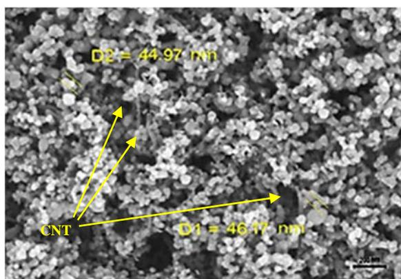
Fig. 2 FE-SEM image of TiO<sub>2</sub>:4%wt.MWCNT thin film morphology
