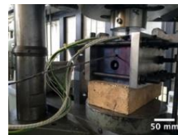
Fig. 1 The photograph of ECAP die used in present study
