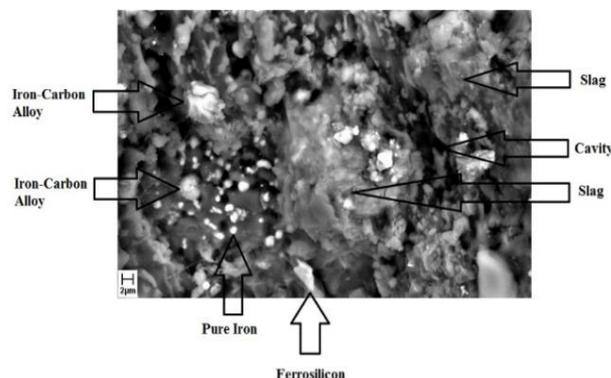
Fig. 4 SEM image of the solidified slag in the back-scattered mode
