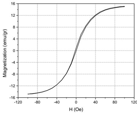
Fig. 2 Vibrating Sample Magnetometer test of CNT0.5 composite
