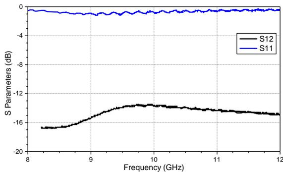
Fig. 3 Shielding Effectiveness of CNT0.1 versus Frequency
