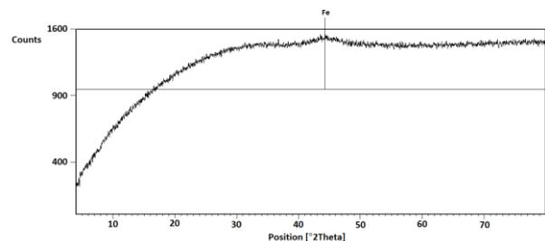
Fig. 1 X-Ray diffraction pattern of Finemet Amorphous Alloy
