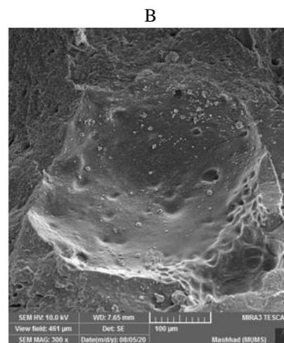
Figure 5: FESEM images of composites after 15 actuation cycles.
