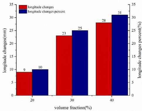
Figure 2 – variation of actuator elongation as a function of ethanol volume.
