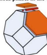
Fig. 2 Schematic illustration of truncated octahedral grains and 3D interfacial regions
