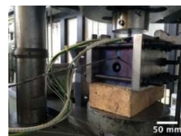
Fig. 1 The photograph of ECAP die used in present study
