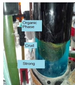
Fig. 3. Crud formation in the stripping stage of spent electrolyte solution (second test)
